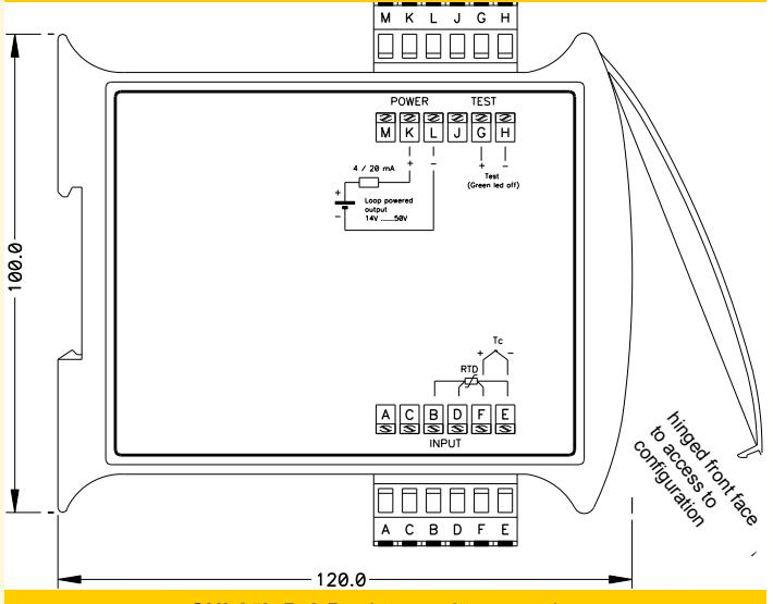
**CNL25igD-2 Dual transmitters version**
